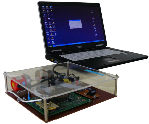
Fig. 2. Electronic measurement system for optical encoder studying.
