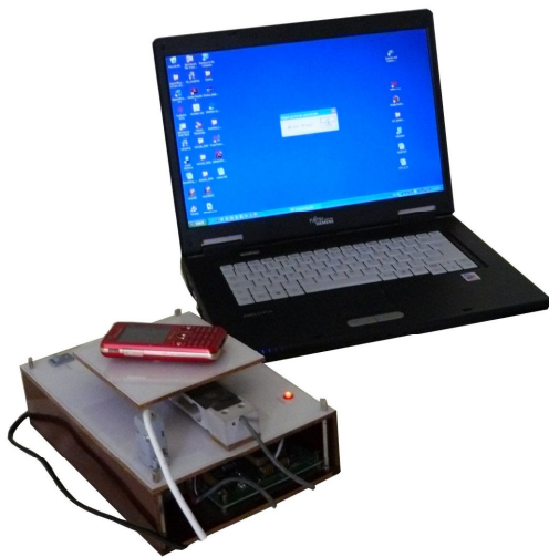
Fig. 6. Electronic measurement system for force sensor studying.
