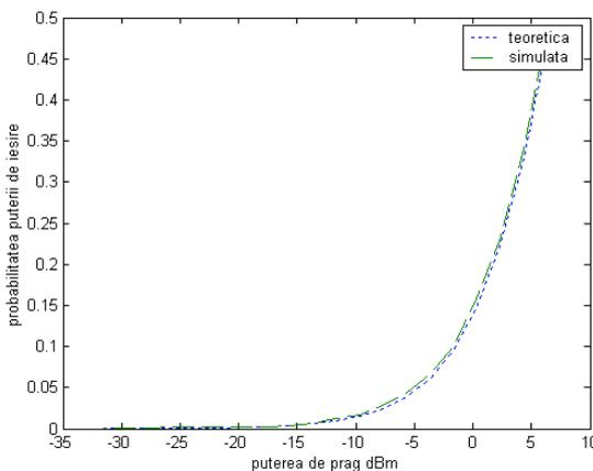
Fig.8 Power outage probability of the envelope using SDR model and 8 bit resolution for the ADC circuit
