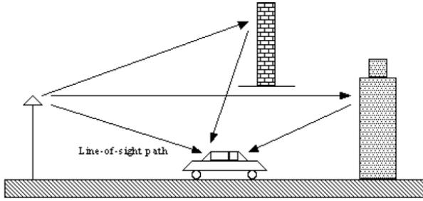
Fig.1. Mechanism of radio propagation in a mobile environment.
