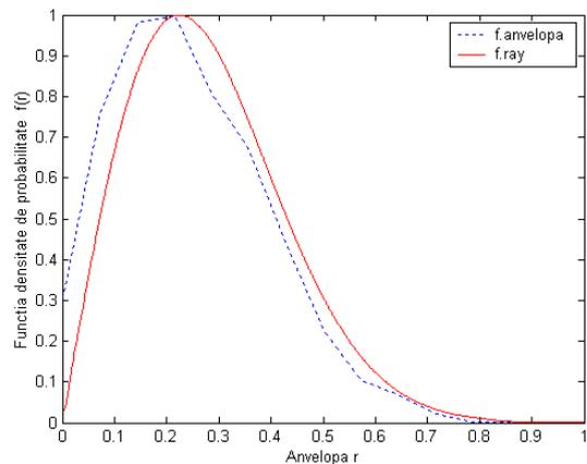
Fig.9 Probability distribution of the envelope using SDR model and 12 bit resolution for the ADC circuit
