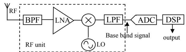
Fig.2 Basic structure of software defined radio
