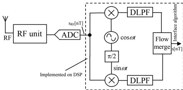
Fig.3 Circuit diagram for a QAM demodulation based on a DSP
