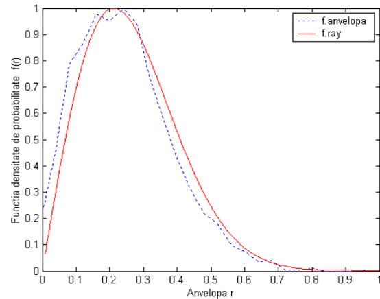
Fig.5 Comparison between the computed probability distribution of the envelope and theoretical Rayleigh probability distribution
