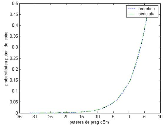
Fig.10 Power outage probability of the envelope using SDR model and 12 bit resolution for the ADC circuit
