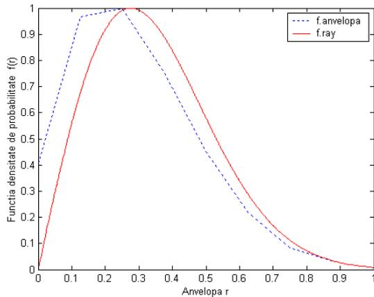
Fig.7 Probability distribution of the envelope using SDR model and 8 bit resolution for the ADC circuit
