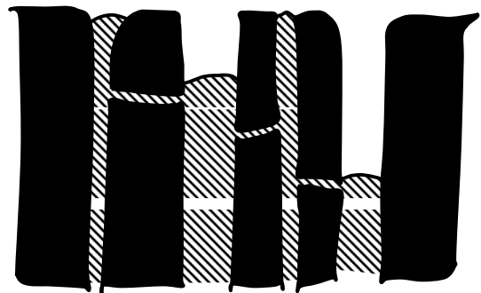
Rate of drying when only the small capillaries are active. Reduced evaporation surface.
