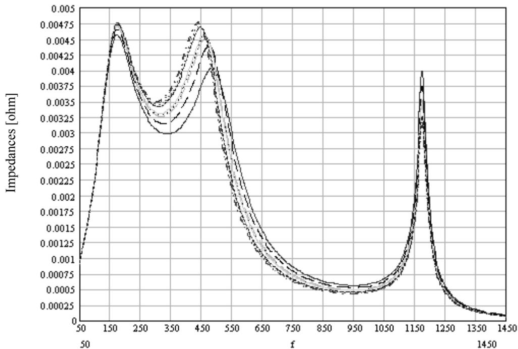
Fig. 4 Frequency characteristics of transfer impedances between nodes of 160, 250, 400, 2x250, 630, 2x400, 1000, 2x630 and 2x100 kVA loads substations and the current source located in a load substation of 1600 kVA.
