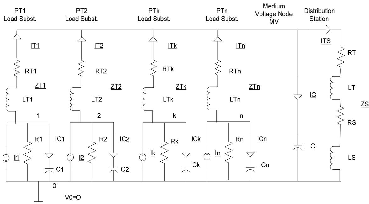
Fig. 1 Equivalent circuit of medium voltage distribution system
