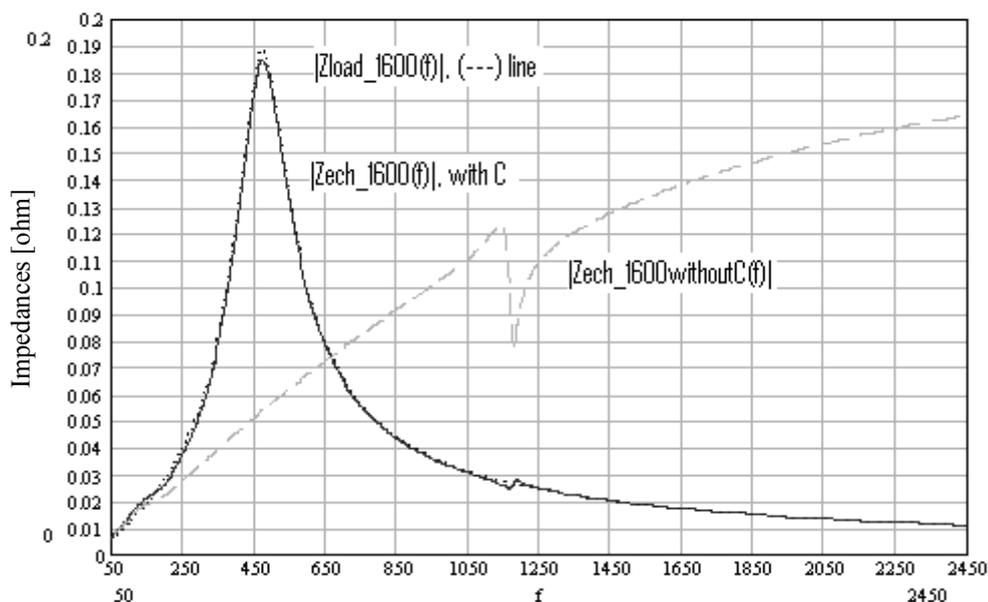
Fig. 2 Frequency characteristics of impedances for a 1600 kVA load substation. Frequency f [Hz].
