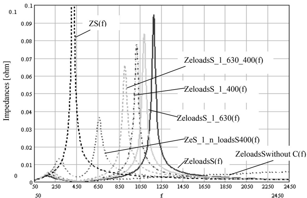
Fig. 3 Frequency characteristics of equivalent impedances seen from medium voltage node MV.
