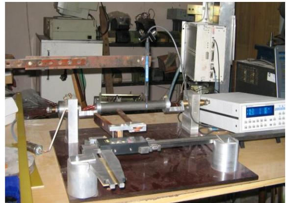
Fig.1 Magnetic induction measuring system
