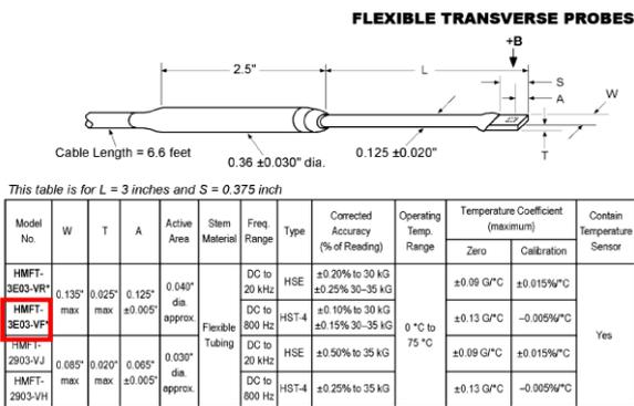
Fig. 3 Catalogue characteristics for transversal Hall probe
