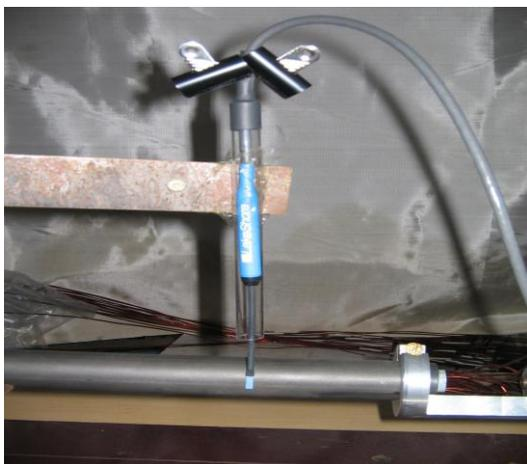
Fig. 4 Hall probe placed perpendicular on the coil's plane
