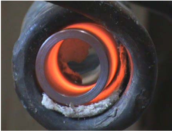
Figure 4. The steel piece inside of the inductor
