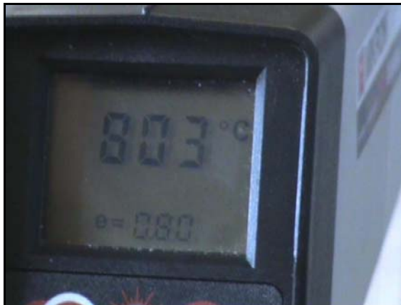
Figure 5. Final temperature of the inductive heating process
