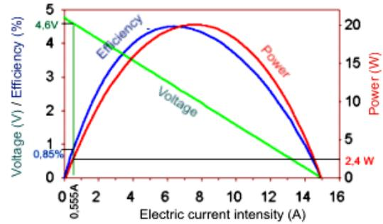
Figure. 6: Power, voltage on load and on module [5]
