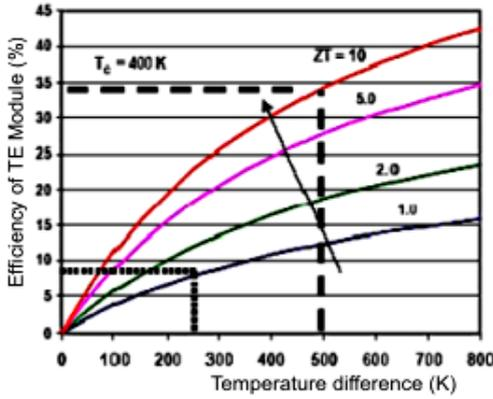
Figure 3 – Thermoelectric module efficiency depending on the temperature difference and figure of merit [3,4]
