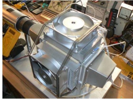
Figure 4: Construction of the thermic recovery of warm gasses and conversion into electric energy
