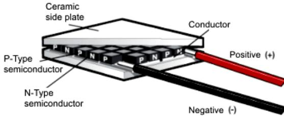
Figure 2: Construction of a Thermoelectric Module [5]
