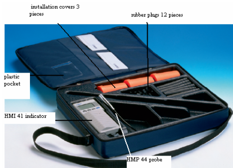
Fig.4: HM 44 set for measuring humidity in concrete
