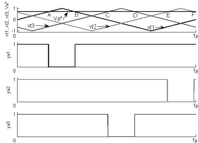
Fig. 3 Phase shift PWM for four level flying capacitor inverter.
