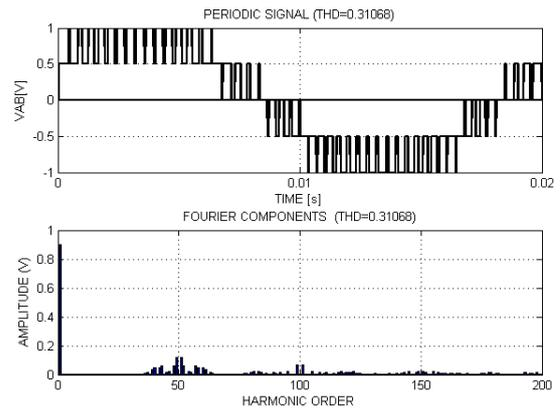
Fig. 10 Phase voltage and fourier components for three level flying capacitor inverter with saw-tooth rotation PWM.
