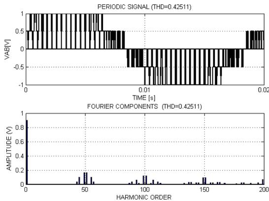
Fig. 8 Phase voltage and fourier components for three level flying capacitor inverter with phase shifted carrier signals.
