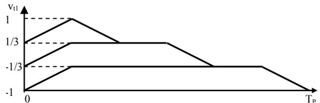
Fig. 5 Carrier signal for a switching cell when carrier redistribution PWM method are used.
