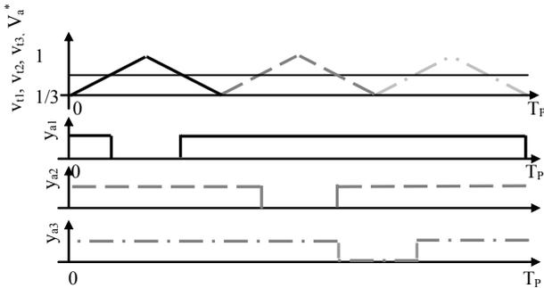
Fig. 7 Carrier redistribution PWM method for four level flying capacitor inverter when modulating signal is between  $[1/3 1]$ .
