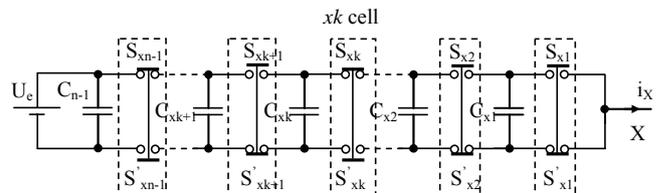
Fig. 2 Inverter leg of flying capacitor multilevel inverter.
