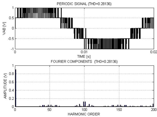
Fig. 12 Phase voltage and fourier components for three level flying capacitor inverter with carrier redistribution PWM.
