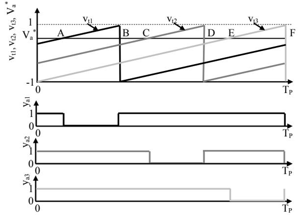
Fig. 4 Saw-tooth rotation PWM method for four level flying capacitor inverter.
