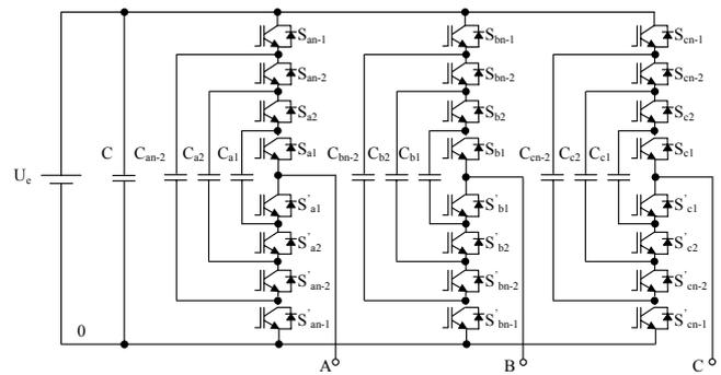
Fig. 1 Circuit diagram of an  $n$  level flying capacitor inverter
