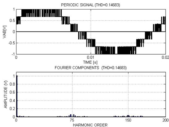
Fig. 13 Phase voltage and fourier components for four level flying capacitor inverter with carrier redistribution PWM.
