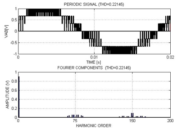
Fig. 9 Phase voltage and fourier components for four level flying capacitor inverter with phase shifted carrier signals.
