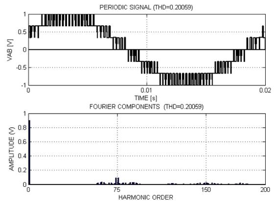
Fig. 11 Phase voltage and fourier components for four level flying capacitor inverter with saw-tooth rotation PWM.
