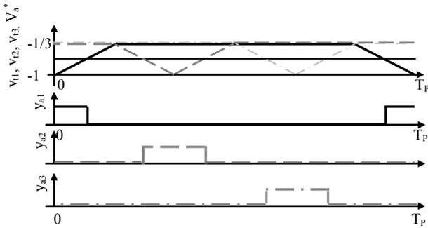
Fig. 6 Carrier redistribution PWM method for four level flying capacitor inverter when modulating signal is between  $[-1 -1/3]$ .
