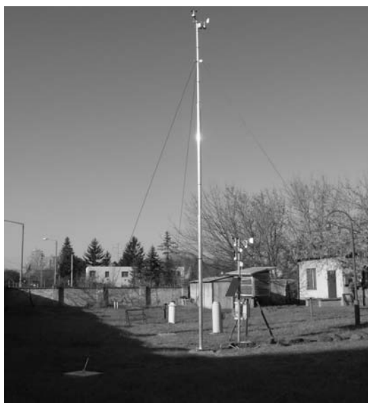
Figure 5 The new automatic urban climate station at the Meteorological Observatory of the University (Source: photos of the author)
