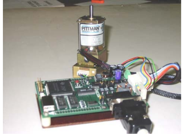
Figure 7. MCK243 target controller with BLDC motor
